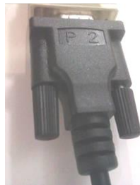
Fig. 3. Picture of one of the four ports of the DB9 male cable, showing the port number.
