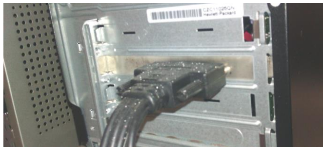
Fig. 2. DB9 male cable attached at the backside of the PC to the PCIe multiport serial board.
